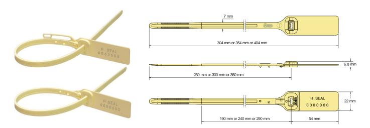
The Acme **H Seal** is a smooth ribbon, pull-tight seal manufactured from Polypropylene material. The design features rolled heat staking technology to secure the metal spring insert to the body, which provides clear evidence of tampering if forced open or cut. The seal can be manufactured with or without gripping spikes and label tag if required. This seal is suitable for many applications where strength is the requirement.
