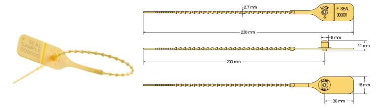
The Acme **F Seal** is a low breaking strength pull-tight seal manufactured from Polypropylene material. The seal can be supplied with a heat rolled over top to prevent tampering by intrusion into the locking head but if tampering is not the main characteristic the seal can be supplied without this added feature. With a 2.6mm diameter ribbon this seal is ideal for applications where there are small sealing apertures.
