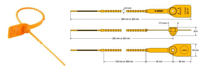
The Acme Griptight Seal is a heavy duty pull-tight seal manufactured from two dissimilar materials. The acetyl insert is durable and will withstand freezing and boiling conditions, whilst the nylon body is flexible for easy use. The design features rolled heat staking technology to secure the insert to the body, which provides clear evidence of tampering if forced open or cut. This seal is suitable for most applications where strength is a requirement.
