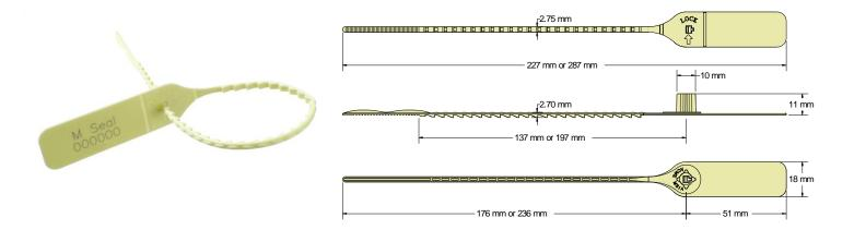
The Acme **M Seal** is a pull tight seal manufactured from Polypropylene material. The locking action is very similar to the tried and tested Minitight (now discontinued) but has the contours of the smooth X Seal. The design offers a cost effective solution for applications where strength is not the primary requirement, but is ideal for use as an indicative seal.
